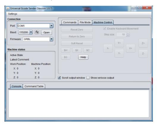
Click the "Machine Control" tab. Select the "Port" number which your Arduino board is attached to. Select 115200 as the Baud rate as this is the speed configured in "GRBL" firmware. Click "Open" button to start the communication for controlling this shield board.
