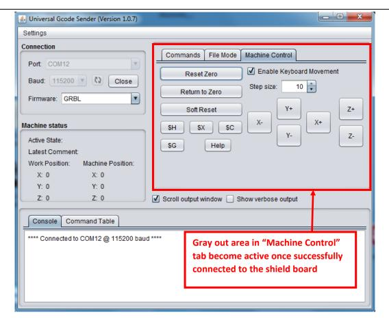
Now, you are ready to control the XYZ stepper motor connected to shield board. Click X+ or X- for example, the stepper motor attached to X terminal will turn in forward or reverse direction.
