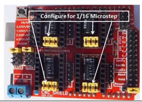
After setting the microstep jumper, you can plug-in A4988 driver boards as shown in the photo below. The photo also shown this CNC sit nicely on top of Arduino Uno board, without any external jumper wires.
