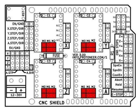
Micro-stepping jumper location, before inserting A4988.
