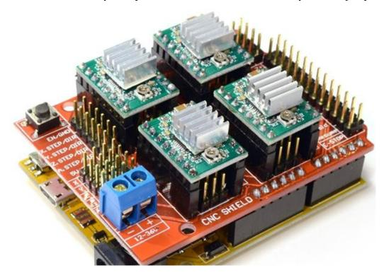
!!! Beware of the orientation of the A4988 driver boards! You will destroy the A4988 driver board if plug-in with wrong orientation.
